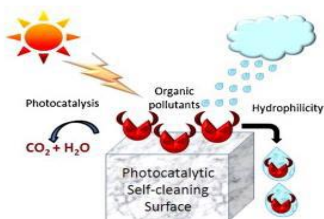
Figure 2.8 Photocatalytic reaction on a self-cleaning surface
