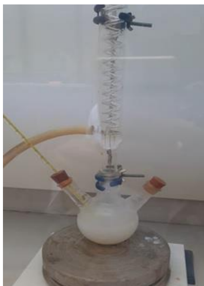
Figure 3.4 Experiment setup for synthesis of the ZnO nanoparticles
