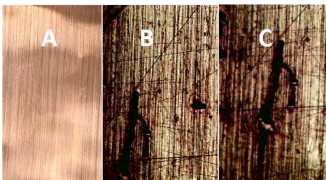
Figure 4.8 Microscopic images of electrodes under air pumping into water compartment, (a) clear copper electrode, (b) corroded copper electrode in water compartment, (c) corroded copper electrode in MO compartment at C=3\text{ g/l} (500x zoom)
