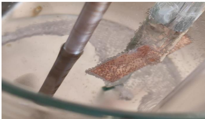
b) The photograph showing air bubbles on the copper electrode (cathode) at N= 450 rpm
