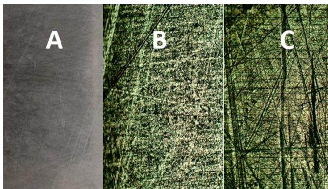
Figure 4.26 Microscopic image of (a) clear stainless-steel electrode, (b) corroded SS electrode of the water compartment, (c) corroded SS electrode of the MO compartment in the presence of agitation in the water compartment at C = 6 g/l (500x zoom)
