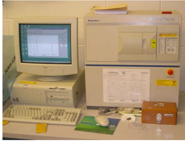
Şekil 3.8 Rigaku Miniflex II Desktop X-Ray Diffractometer
