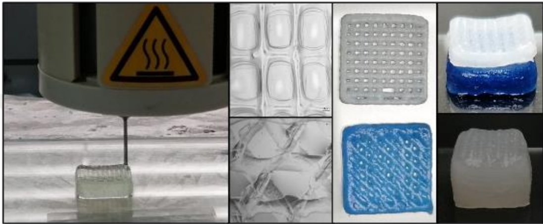
Figure 4. 20 3D printing of cartilage and bone scaffold in grid and snowflake pattern, respectively.
