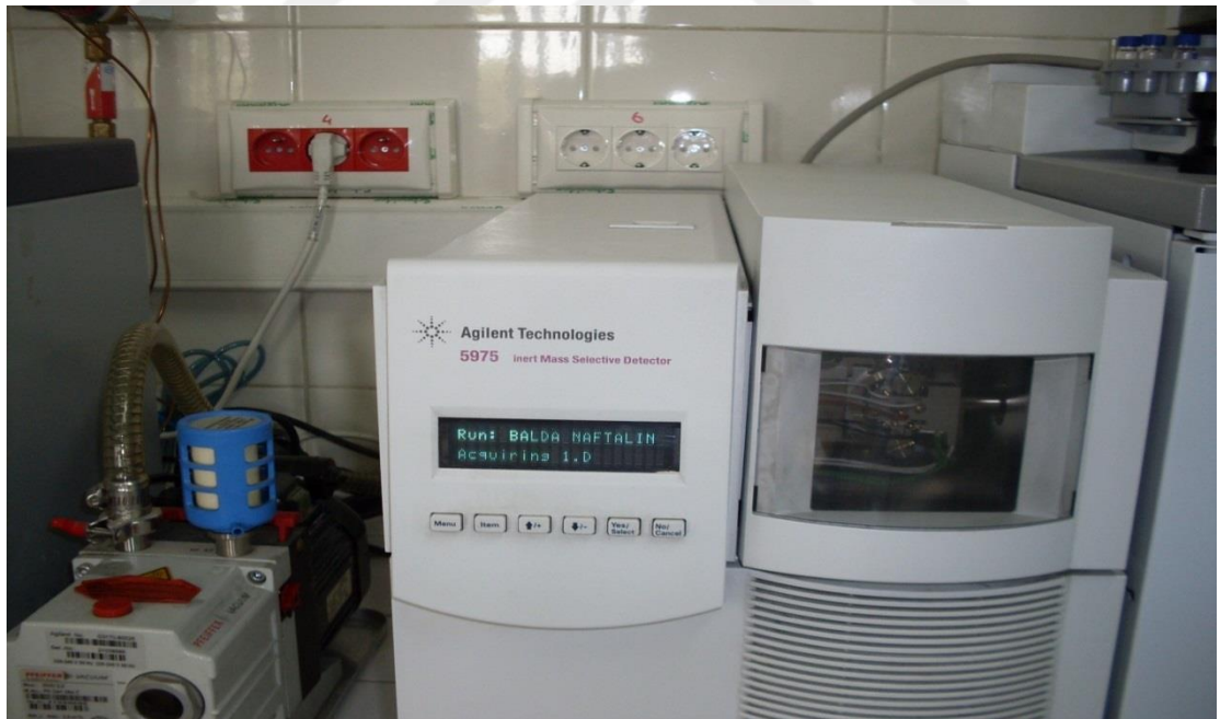
Şekil 2.2. Kütle Spektrometresi (MS) Agilent Techonologies 5975 Mass Selective Detector.
