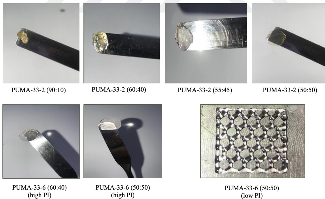
Figure 4.5 Optimization of PUMA blend hydrogel formation in the presence of EY, TEA and VP using UV light. PI: Photoinitiator
